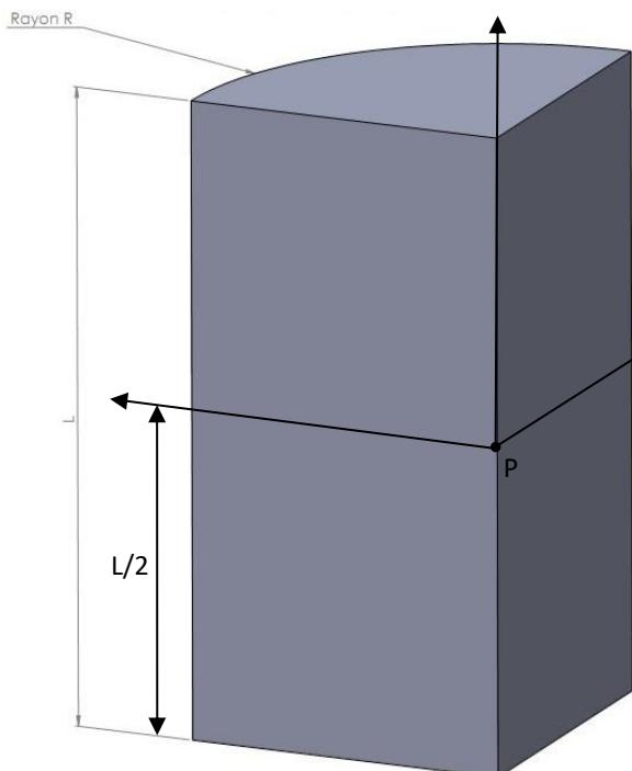
$$\bar{\bar{I}}(P, S) = m \begin{bmatrix} \frac{R^2}{2} + \frac{L^2}{12} & -\frac{R^2}{2 \cdot \pi} & 0 \\ -\frac{R^2}{2 \cdot \pi} & \frac{R^2}{2} + \frac{L^2}{12} & 0 \\ 0 & 0 & \frac{R^2}{2} \end{bmatrix}_{(\bar{x}, \bar{y}, \bar{z})}$$
